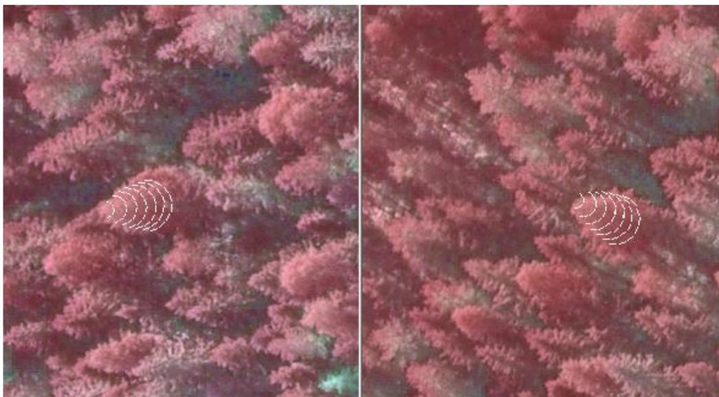
Figure 7: 40-year-old birch as seen in a stereo pair (UltraCam D, 1 km). The fitted crown is superimposed in the images. The XY-offsets in treetop positions and asymmetry of crowns (non circular) (in addition to image orientation errors) caused undoubtedly some errors when crowns were projected to the different images. (Source: I. Korpela)
